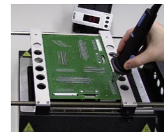
Lead-free desoldering with heating plate (IRHP 200)
