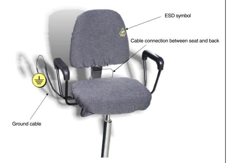
Made of gray conductive woven fabric, the dissipative chair covers are designed to make a conventional padded factory chair more suitable for use in EPA.
